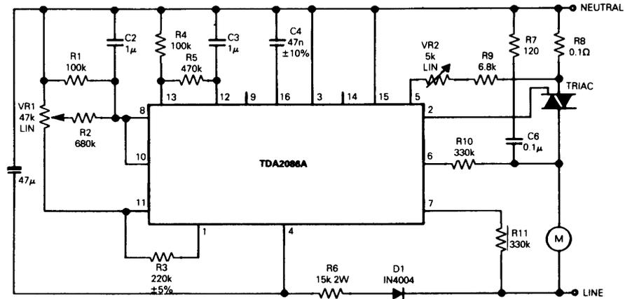
Figure 12 Optical feedback application
