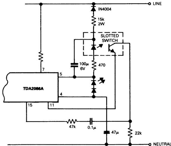
Figure 13 Current limit foldback, method 1
