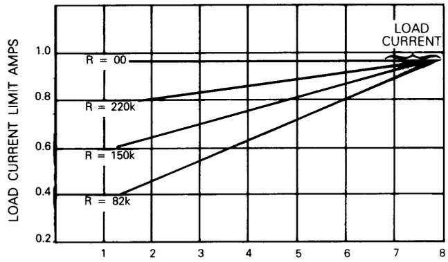
Figure 14 Current limit foldback, method 2
