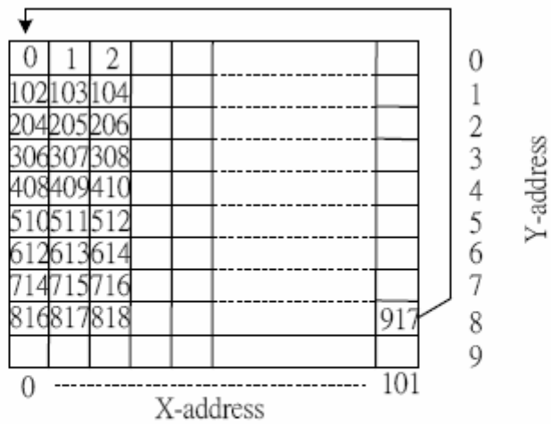
Fig.14 sequence of writing data bytes into RAM with horizontal addressing
