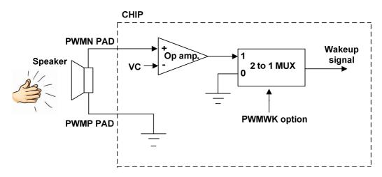
Wakeup control block diagram and speaker trigger application circuit
