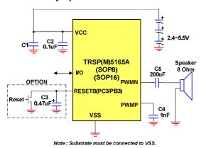
Figure 15. DAC Applications circuit -1
