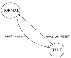
Figure 2: Clock Operation Mode
