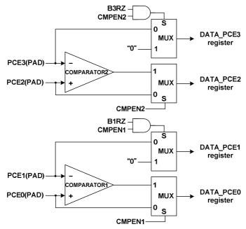
Figure 11. Port PCE mode 2 block diagram
