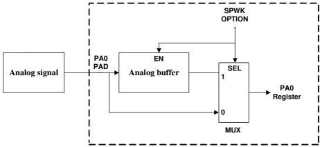
Figure 6. PA0 analog input structure
