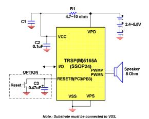
Figure 14. PWM Applications circuit -2
