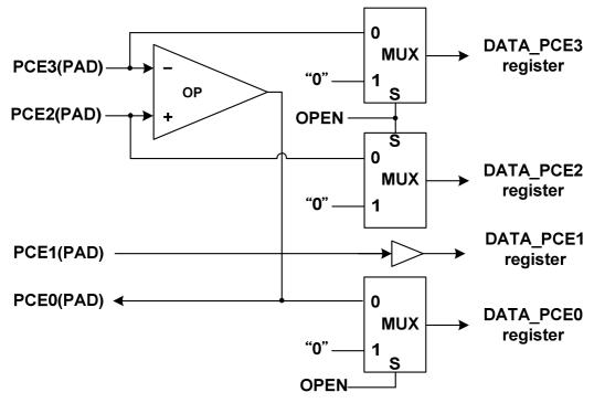
Figure 10. Port PCE mode 1 block diagram
