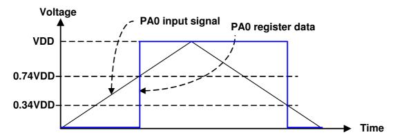
Figure 7. PA0 input signal and PA0 register data
