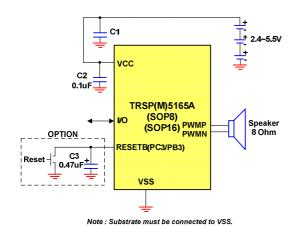
Figure 13. PWM Applications circuit -1
