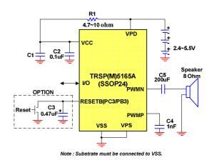
Figure 16. DAC Applications circuit -2
