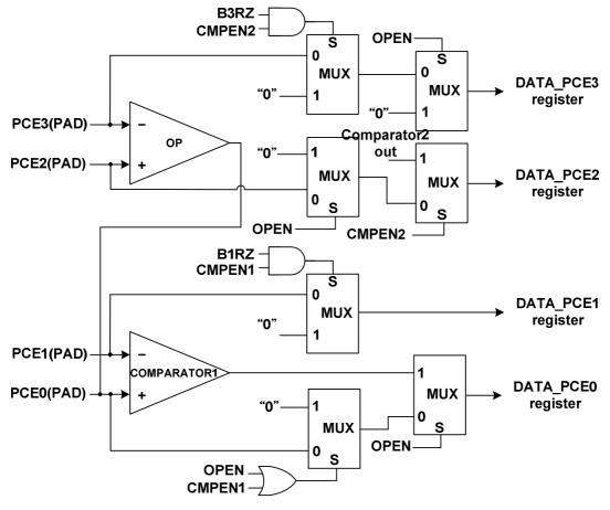
Figure 12. Port PCE mode 3 block diagram
