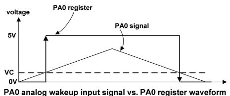
Figure 9. PA0 register waveform
