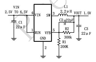
Figure 1. Basic Application Circuit with APS2415 adjustable version
