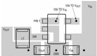
Figure 5. APS 2415 Fixed output Suggested Layout
