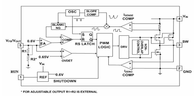
Figure 3. APS2415 Block Diagram
