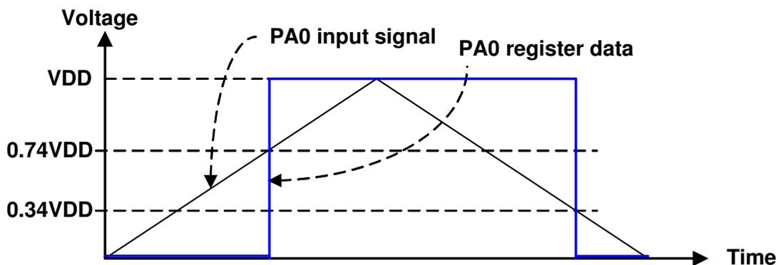
Figure 7. PA0 input signal and PA0 register data
