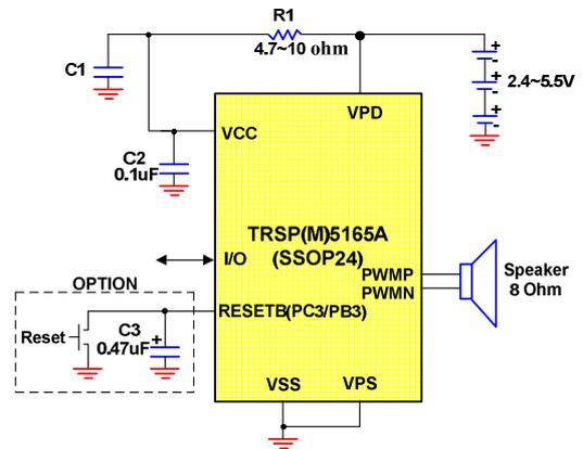
Note : Substrate must be connected to VSS.
