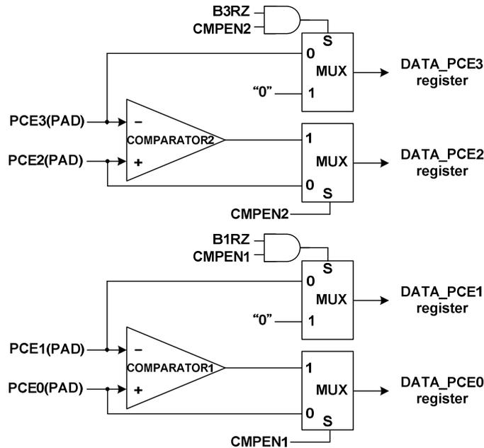
Figure 11. Port PCE mode 2 block diagram
