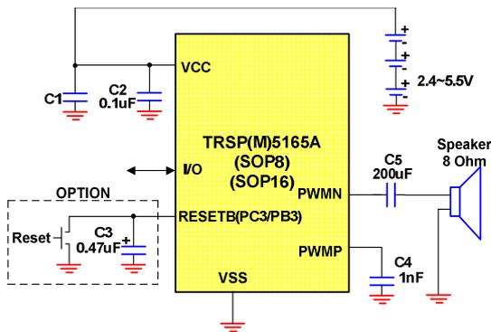
Note : Substrate must be connected to VSS.
