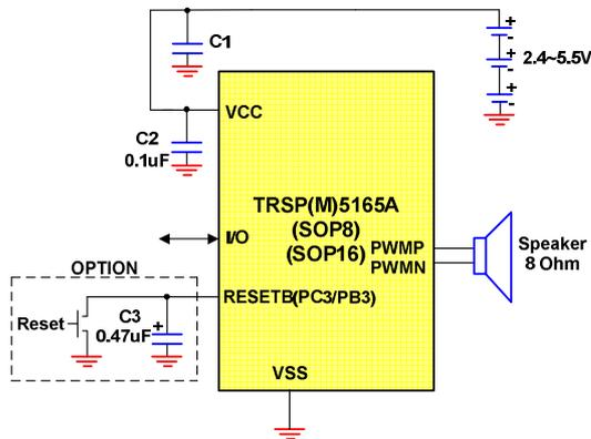
Note : Substrate must be connected to VSS.
