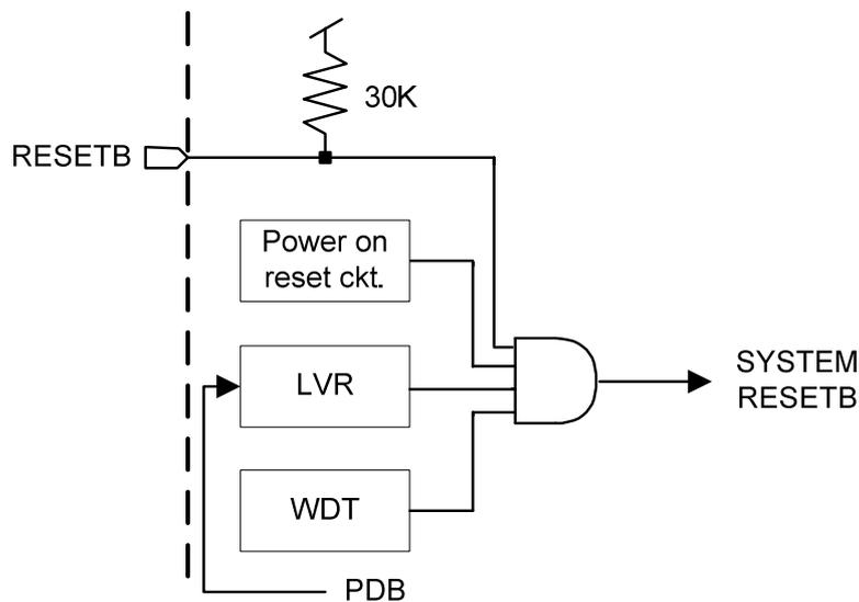
Figure 5: Reset structure
