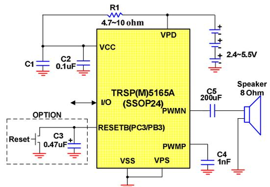
Note : Substrate must be connected to VSS.
