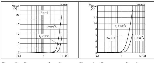
Figure 5. Collector-source On voltage Figure 6. **Collector-source On voltage**
