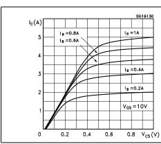
Figure 1. **Output characteristics**
